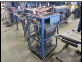
Shop built bender w/ hydraulic power pack
